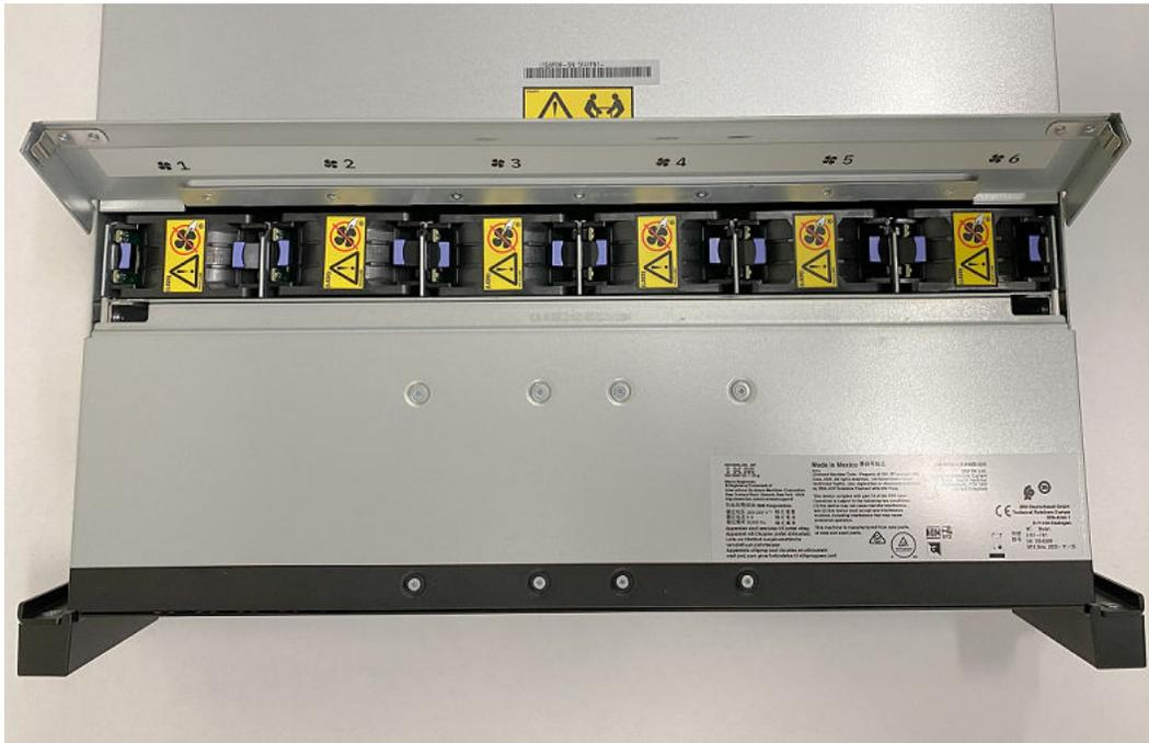
Figure 76. IBM Elastic Storage System 3200 fan LEDs
