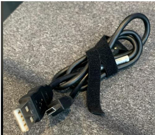
Figure 94. Serial (USB mini-B) to USB cable
