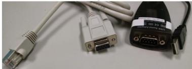
Figure 89. RJ45 to serial cable and USB to serial cable
