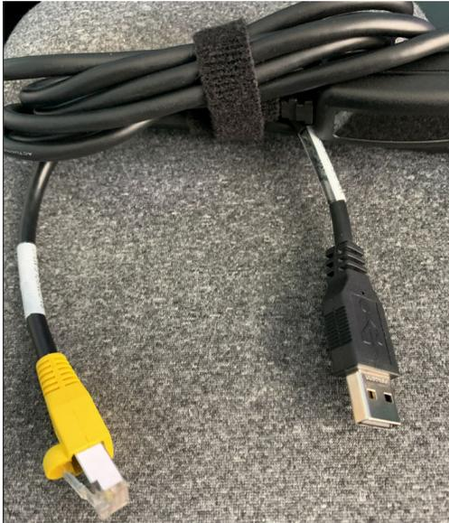
*Figure 95. POWER9 EMS (serial to USB)*
