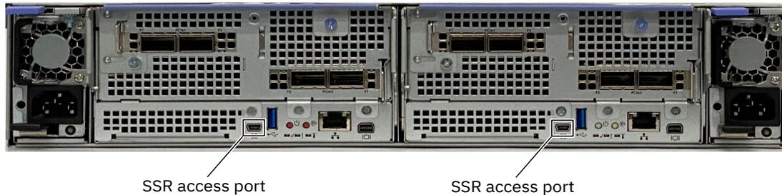
Figure 50. SSR access port/mini USB
