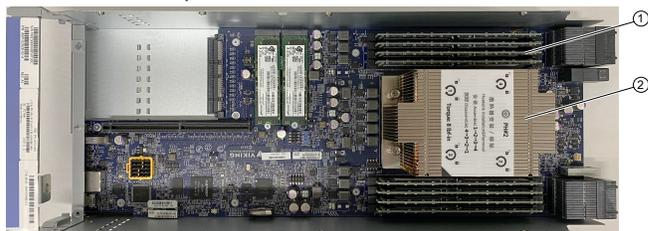
Figure 10. Location of CPU and DIMM slots within the server canister
