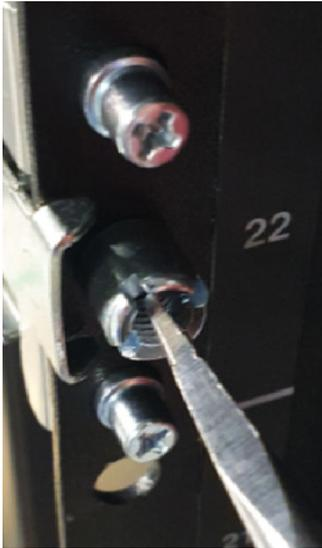
*Figure 27. Securing the front of the rails*
